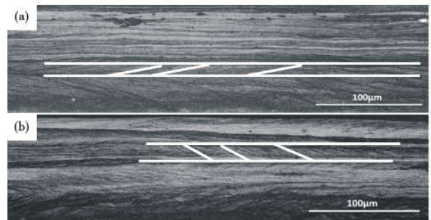
图 5 3% Si 钢冷轧板组织:(a) 薄带铸轧;(b) 常规流程 Fig. 5 Microstructure of cold rolling plate of 3.0% Si steel: (a) thin strip casting rolling process; (b) routine process
